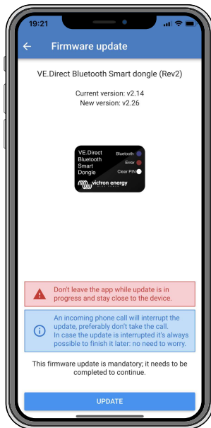
Screenshot dongle firmware update using VictronConnect
