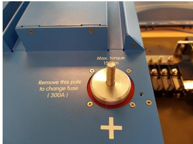
2. Lift the aluminum battery pole;
